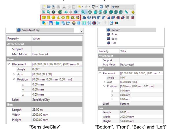
**Hint:** Since the cubes we created for the "Bottom", "Front", "Back" and "Left" objects have the same dimensions and positions, you can create one cube for "Front", for example, then go to "Edit" on the menu → Duplicate selection.
