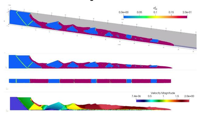
In this project, you will apply a softening plasticity model to analyse retrogressive failure.
